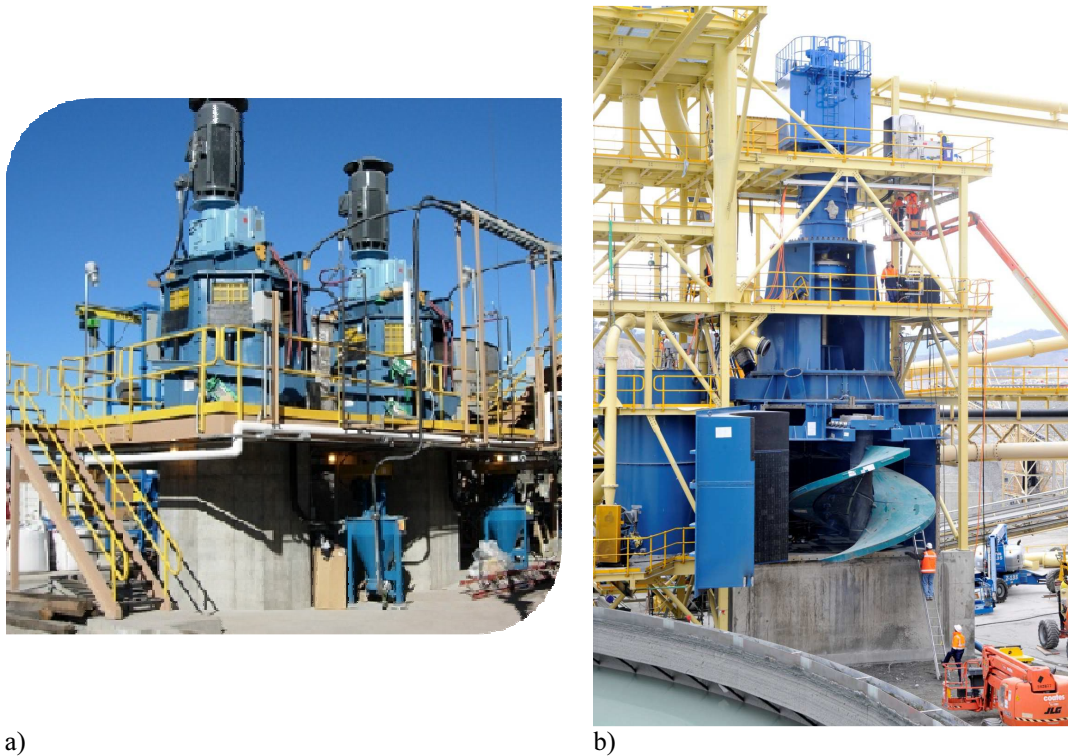
Figure 3 – Application of Metso’s a) Stirred Media Detritor (SMD) and b) VertiMill® in mineral processing plants (with permission from Metso Minerals)
