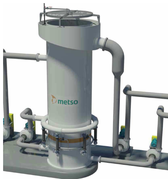
Figure 4 – Schematic of the Microcel™ column flotation cell (with permission from Metso minerals)
