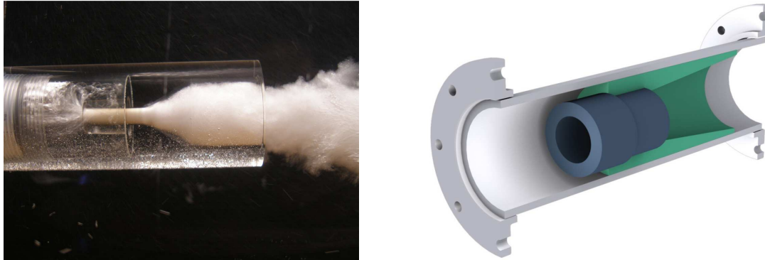
Figure 5 – A model of the CavTube™ sparging system (with permission from Eriez)
